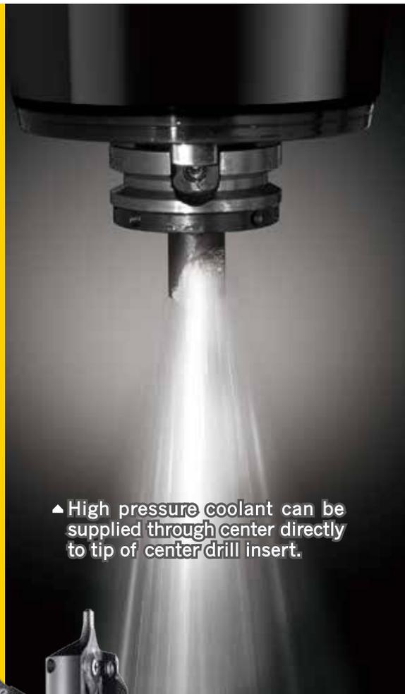
▶ High pressure coolant can be supplied through center directly to tip of center drill insert.
