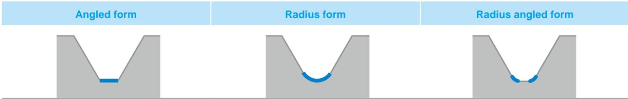
**Unlimited variations :** The X060 insert will be designed based on your specific application of angle, width, depth and radius.
